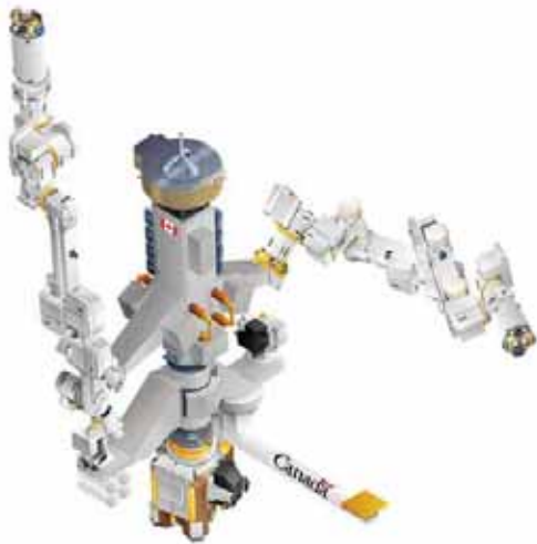
SPDM bi-arm system[MD Robotics] 3.5 m class arms
