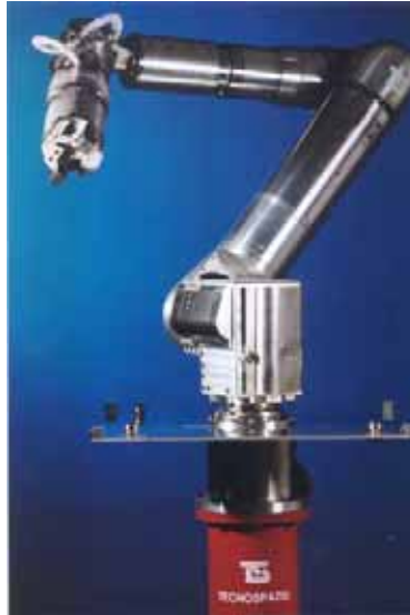
SPIDER Arm [Galileo Avionica] ASI Contract 1.5 m class arms
